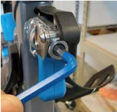
3. Press the adjustment knob to its end-of-stroke position against the return spring
