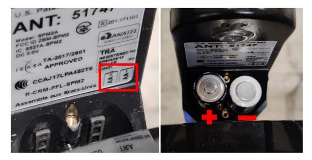
The batteries should slide into place smoothly. If the batteries won't reinsert without force, remove them double-check that there is not too much tape applied.
